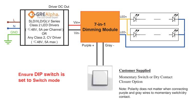
\*\* Note alternate simple on-off operation:
